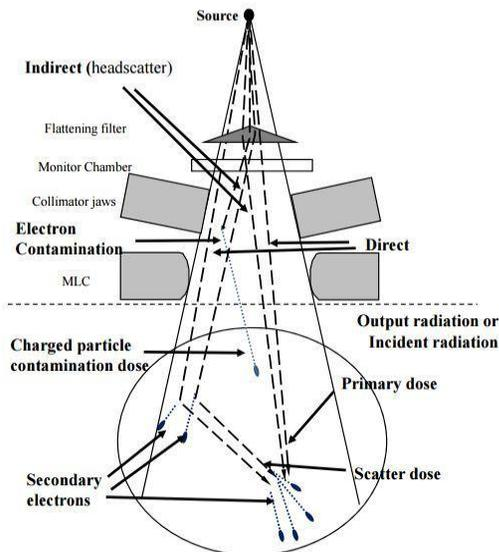
**Fig. 2.** Internal Construction of LINAC [11]
