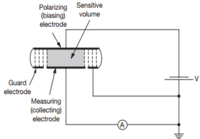
**Fig. 4.** Circuitry of a dosimetry system which is based on ionization chamber [12]
