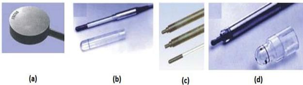
**Fig. 3.** Examples of some ionization chambers which are used in radiation therapy[12]: (a) Parallel plate Roos type electron-beam ionization chamber; (b) Farmer type cylindrical chamber with a Cobalt-60 buildup cap; (c) Cylindrical ionization chambers (for relative dosimetry); (d) Pinpoint mini-chamber and Cobalt-60 buildup cap.
